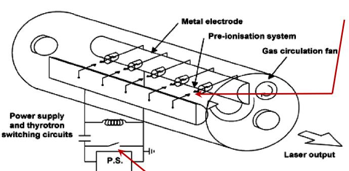
Preionization is actually quite important. It is a discharge that occurs before the main discharge, emitting UV light. This light ionizes some species throughout the gas, making sure the main discharge fills the space between electrodes. No localized lightning bolts!
