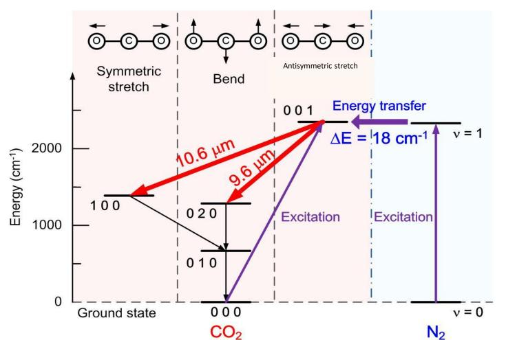
Relatively to other gas phase lasers, this is a highly efficient laser, converting 10-20% of the electrical power into laser energy.
