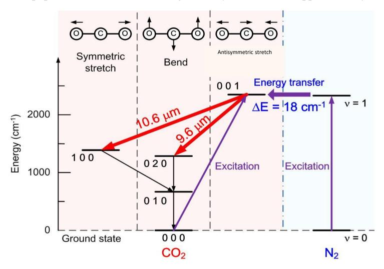
To maintain the population inversion, the population in the lower level of the transition must be depleted quickly. Collisions with helium atoms are effective in dropping the  $CO_2$  molecules in the v=1 symmetric stretching level to lower levels, allowing the population inversion to be maintained.
